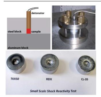
Fig. 2 Small-scale reactivity test of TKX-50, RDX and CL-20. Above pictures: test setup for the SSRT. Below: dented aluminium blocks after initiation of the explosive with a commercial detonator.
