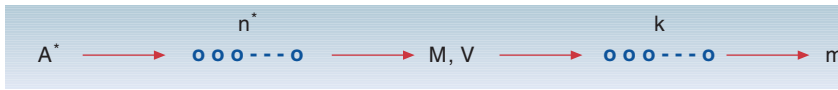
Figure 28 A fictitious equivalent group for generation of a given overflow M, V
