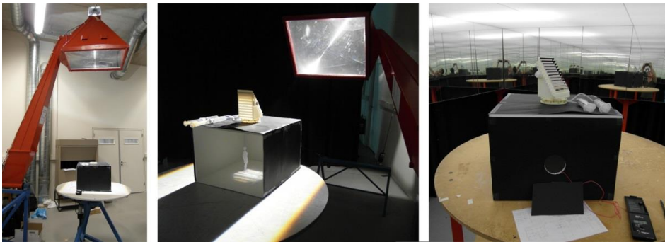
Figure 106. Left: Solar Simulator at a 90° altitude (Test 1). Middle: Solar simulator inclined at a 30° altitude (Test 3). Right: Set up for Test 4, using the Artificial Sky Simulator.
