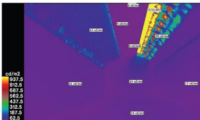
Figure 126. Daylight simulation 21.06., clear Sky with sun, 14:00, with and without reflectors
