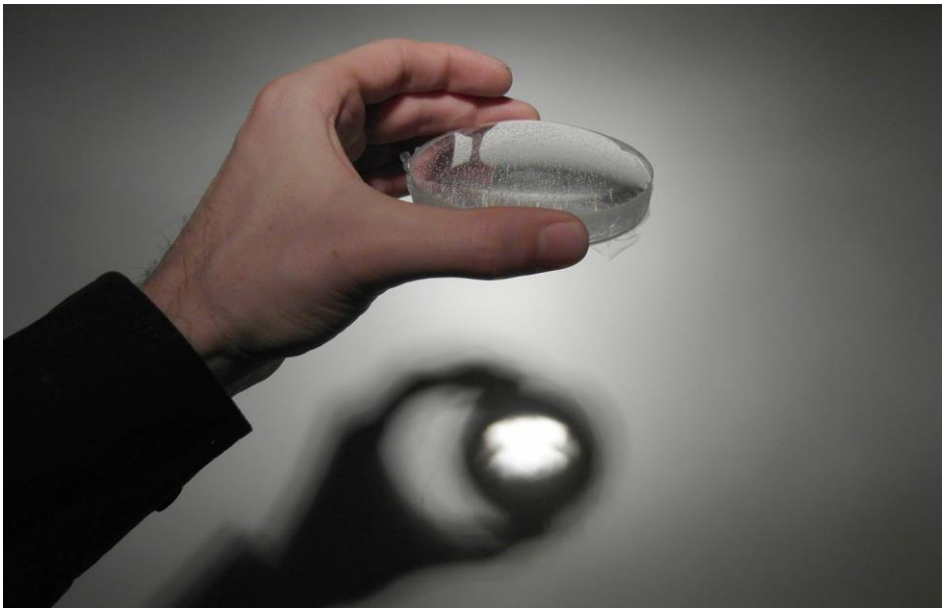
Figure 98. First prototype consisting of transparent petri dish and clear plastic wrap filled with water
