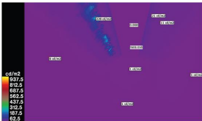
Figure 128. Daylight simulation 21.06., clear Sky with sun, 18:00, with and without reflectors
