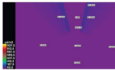
Figure 129. Daylight simulation 21.06., overcast sky, 10:00, without and with reflectors
