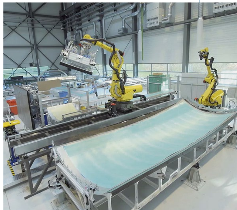
Figure 5 Test cell for the automated lay-up of FML (© Premium AEROTEC)
