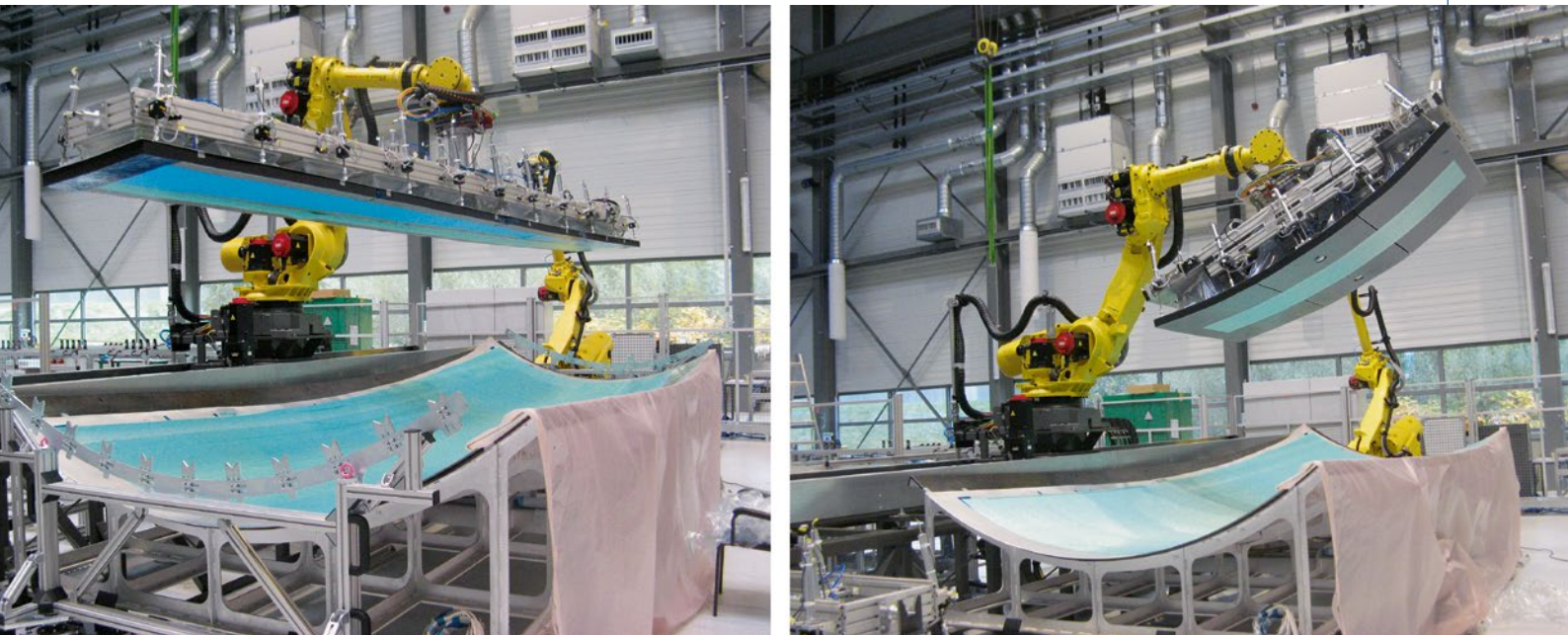
Figure 7 Laying up glass fibre prepreps for FML (© Premium AEROTEC) (© Premium AEROTEC)
