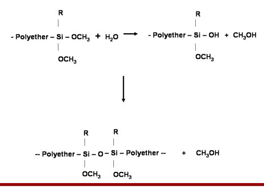
Similar to other sealants, MS polymers can be formulated with various plasticizers, fillers, and other additives to provide a wide range of properties depending on the application. Single-part formulations are most common, but two-part formulations are also possible.
