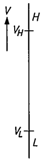
Fig. 3. In digital circuits, in the steady state the output voltage is in one of the two ranges indicated by L and H. The signal temporarily enters the transition range only during the transition from L to H or vice versa.
