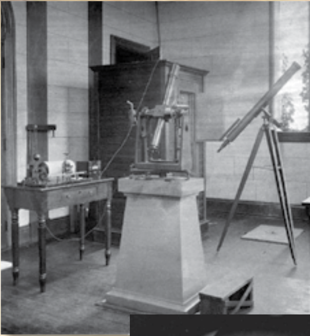
Drum Chronograph, Buff & Berger Meridian Circle on pier and 4" Clark Comet Seeker Telescope
