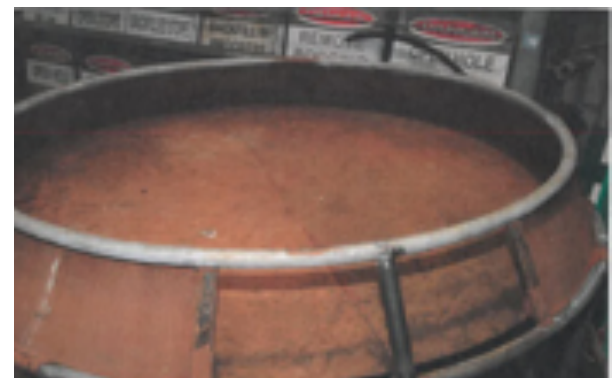
Steel cables are delivered to site in coils (top). Stan Butterworth's cradle structure reduces the risk of personnel being struck by a rapidly uncoiling cable when the ties holding it together are cut.
