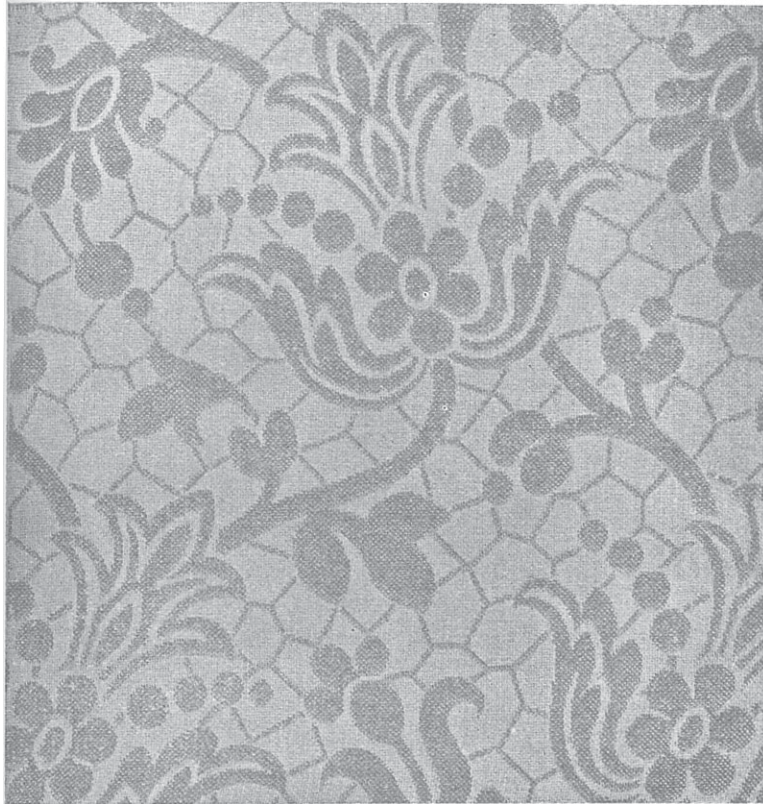
FIG. 297.—DOUBLE-PLAIN WOVEN SPECIMEN.
