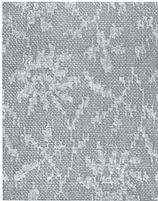
FIG. 299.—REVERSIBLE FIGURED TYPE—SILK AND COTTON YARNS.
