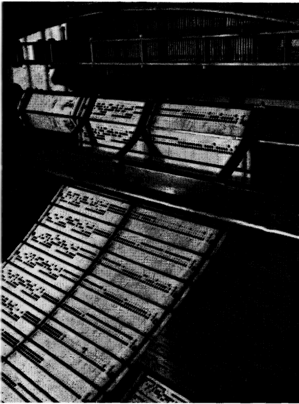
The Jacquard is the "brain" of the machine. The numbers on the draughtsman's chart are translated into a series of holes punched in Jacquard cards, like the holes in a player-piano roll. The cards are laced together to form an endless band and placed under a set of steel rods. As each card rises all rods not directly under holes are pushed up. This motion determines the pattern.
