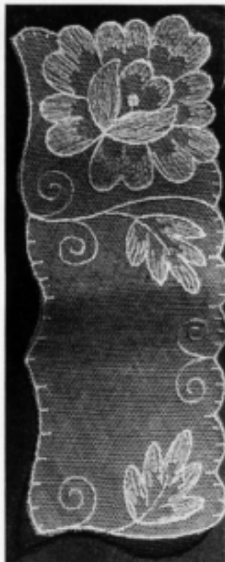
Here is a close-up of the embroidered net which is being produced on the embroidery machine above. The actual design, enlarged six times on draught paper, is being followed by the pantograph operator at left. This piece of fancy net will form part of the trimming of a linen handkerchief.
