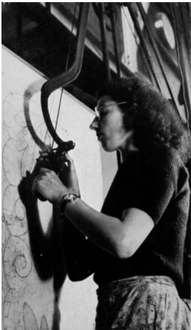
The pantograph plays a vital role in creating the design in Schiffli embroidery. A much enlarged plan of the design on draught paper is followed in outline by the operative with a needle tracer. Any movement of the needle is duplicated in the machine by a change in position of the fabric base on which the design is being reproduced.
