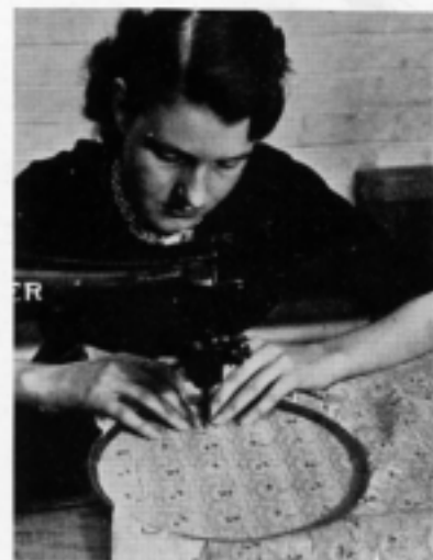
From the embroidery machines the goods pass to the examination tables where skilled machinists make good any flaws in the design. Detailing missed by the machine can be put in and matched perfectly to the pattern. Multi-colour embroideries are receiving attention in this picture.
