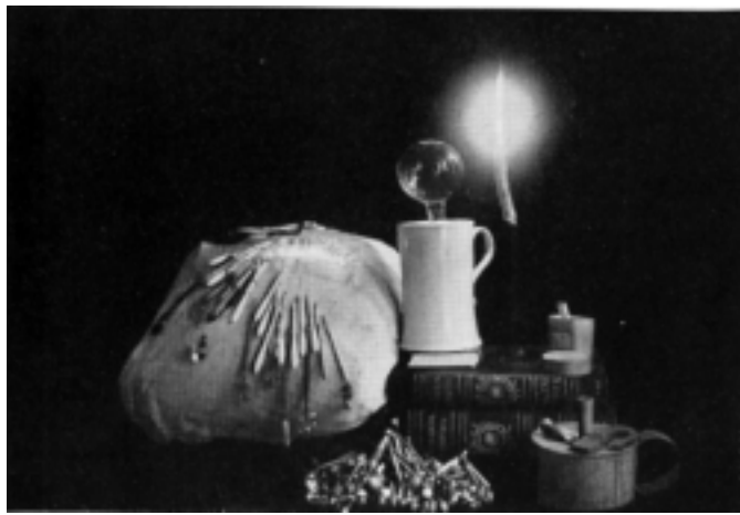
Implements of the pillow lace maker: bobbins, rushlight and reflector. The pattern is pricked on a parchment pattern which lies on the surface of the pillow and the lace is worked over it.
