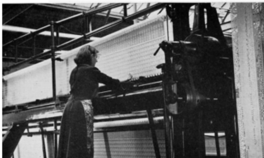
More modern than the pantograph is the automatic Jacquard attachment. Its action is to move the fabric in various directions as the design takes shape, so that the needles form a continuous pattern.
