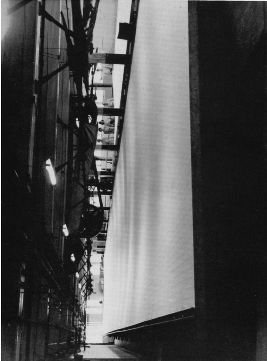
Dressing frame with web in place
