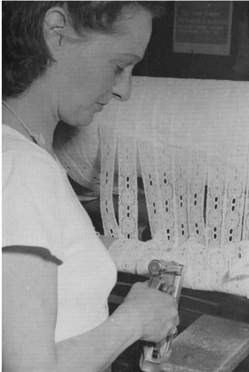
Fastening the bands to cardboard tubes
