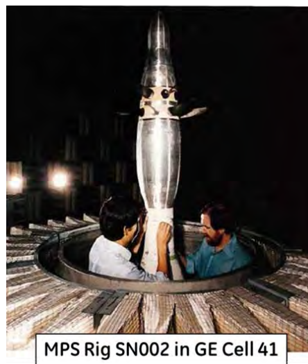
Figure 2: GE Cell 41 model-scale open rotor rig.
