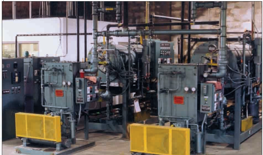
Fig. 1 — An endothermic gas generator, left, and two exothermic gas generators, right. Photos courtesy Seco/Warwick Corp., Meadville, Pa. ( www.secowarwick.com ).
