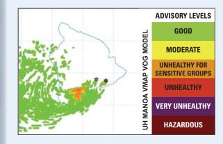
The Vog Measurement and Prediction Project (VMAP) uses estimates of volcanic emissions along with wind forecasts to predict concentrations of sulfur dioxide gas (SO<sub>2</sub>) and sulfate (SO<sub>4</sub>) aerosols. The colors on the map are correlated with the Hawaii State Department of Health advisory levels (weather.hawaii.edu/ vmap).
