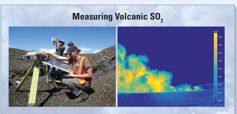
Two paired of cameras sensitive to ultraviolet light (left) image the eruption plume as it rises from the lava lake. The analyzed image from October 17, 2016 (right) displays warmer colors for higher SO, concentrations in the plume. Photograph by T. Elias, USGS.
