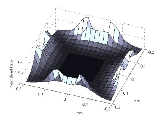
3(b) Normalised dielectrophoretic force across the region defined by the electrode tips, and  $3\mu m$  above the electrode plane.
