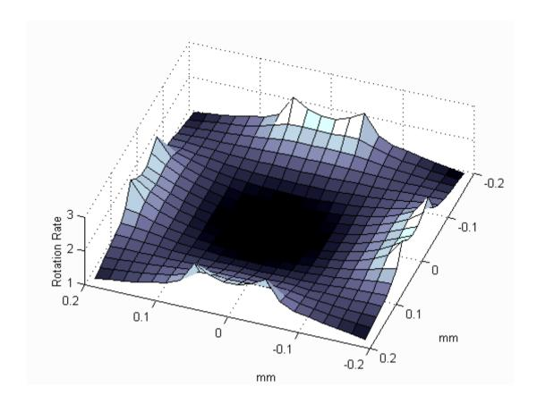
Spatial variation of the field factor  $E^2_{eff}$  ( $V^2\mu m^{-2}$ ) across the region defined in Figure 1, as generated by a polynomial electrode array. Note the degree of variation in field factor (and consequently induced torque) between the centre and edge of the array.
