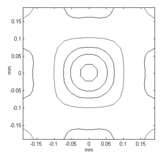
3(a) Variation in torque from the value at the centre of electrode chamber. Lines indicate (from centre) the limits of 1%, 5%, 10% and 20% variation. Variation in excess of 50% is visible near electrode tips (at the centre of each edge). A sharp decline in rotational torque towards the corners of the box visible in the corners of the box, where the torque drops *below* 20%.
