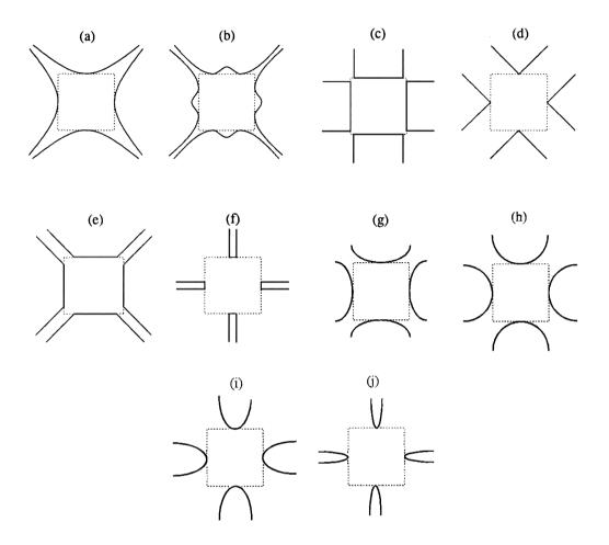
Schematics of the electrode designs studied here. (A) polynomial (b) bone (c) square (d) pointed pyramidal (e) truncated pyramidal (f) pin (g) oblate ellipse (h) circular (i) prolate ellipse, (j) narrow prolate ellipse.
