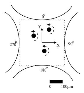
Schematic of a polynomial electrode array, as used for Electrorotation (ROT).
