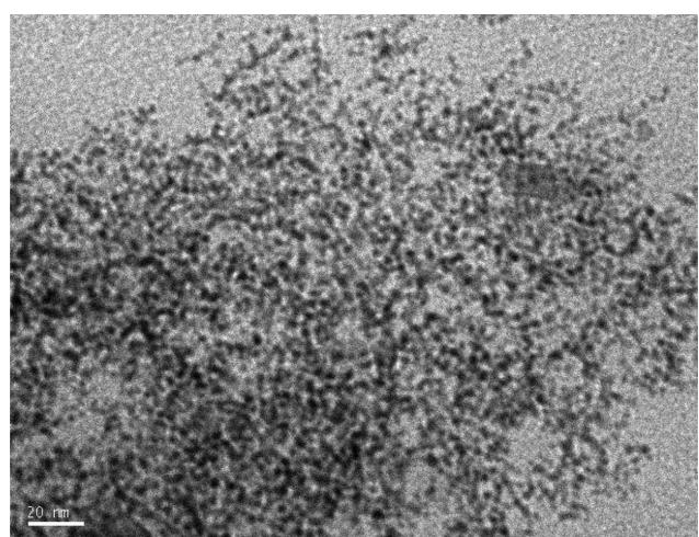
**Fig. 2.** TEM image of as-synthesized FePt nanoparticles.
