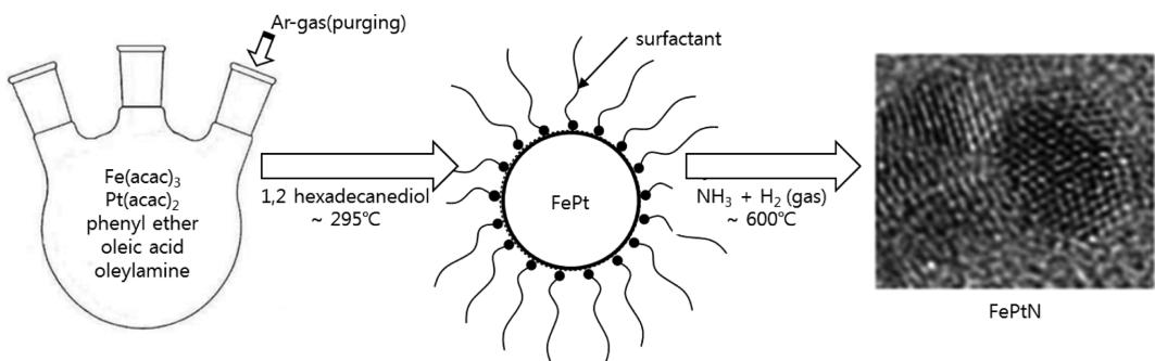
**Fig. 1.** Schematic diagram of thermal decomposition and mixed-gas nitridation.
