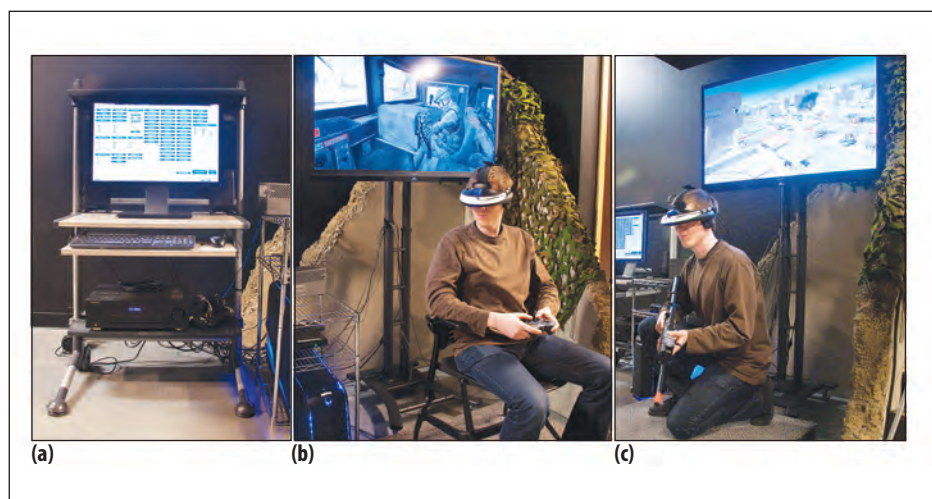
Figure 2. Sample Bravemind system components. (a) A clinician interface for modifying VR settings in real time to match user experiences. (b) VR head-mounted display and traditional gamepad used by a seated participant in a driving scenario. (c) Rifle-mounted mini-gamepad used in a walking scenario.
