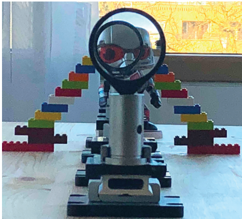
Figure 5. Front view through Lens 4 of the invisibility cloak in figure 4. Notice that the green Lego block joining the two sides of the bridge can not be seen and Giant-Man's head and eye are visible. For this image other blocks are obscured by the lens holders.
