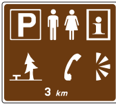
Advance sign for facilities in lay-by
