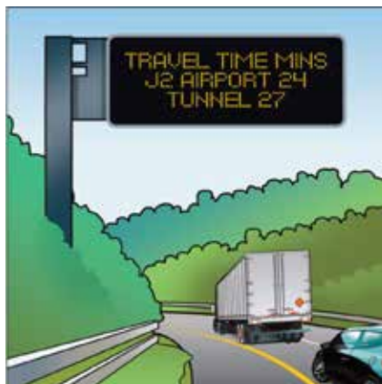
Typical LED VMS
