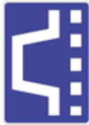
Emergency (Tunnel) Lay-by
