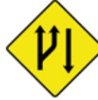
Start of a climbing lane
