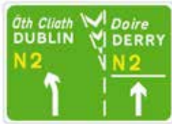
Lane destination sign
