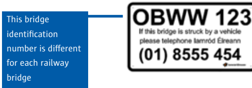
Example Railway Bridge Identification Plate
