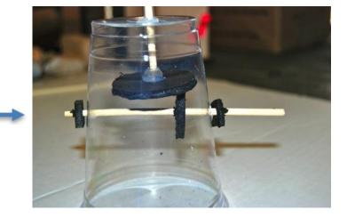
Slide a skewer through a side hole, through a circle, and then through the 2<sup>nd</sup> side hole. This is the crankshaft.
