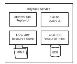
**Figure 4. Simple Standalone Deployment**
