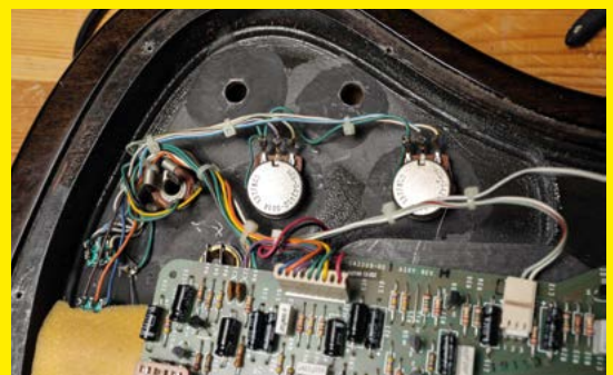
FITTING THE ELECTRONICS INSIDE NECESSITATED ROUTING AN UNUSUALLY LARGE HOLE IN THE BACK
