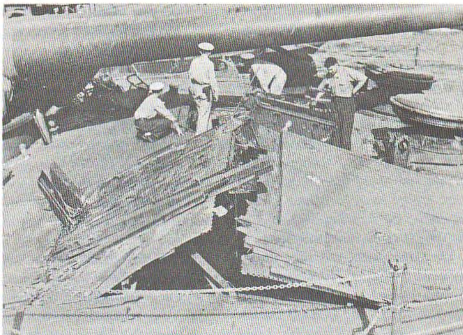
USS Nevada, showing bomb rupture on bow, forward of turret I.
