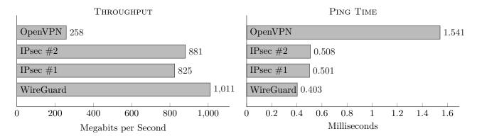
For both metrics, WireGuard outperformed OpenVPN and both modes of IPsec. The CPU was at 100% utilization during the throughput tests of OpenVPN and IPsec, but was not completely utilized for the test of WireGuard, suggesting that WireGuard was able to completely saturate the gigabit Ethernet link.
