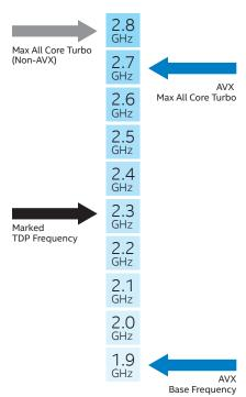
**Figure 2.** The new Intel® Advanced Vector Extensions (Intel® AVX) instructions could operate at or below the marked TDP frequency, while still providing up to two times the floating-point throughput.
