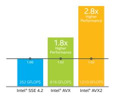
**Figure 1.** Measuring performance on the same processor using Linpack\* benchmarks shows substantial increases from Intel® Streaming SIMD Extensions 4.2 (Intel® SSE 4.2) to Intel® Advanced Vector Extensions (Intel® AVX) and from Intel AVX to Intel® AVX2, with up to 2.8x the GFLOPS throughput when comparing Intel SSE 4.2 to Intel AVX2.<sup>2</sup>
