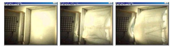
Blast Shield deploying under a blast load catchers fragments and debris.
