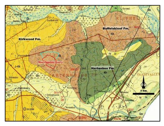
Figure 6. Geology of the area. Extract of 1:50 000 Geological Series 3422AA. Geological Survey, Department of Mineral & Energy Affairs.
