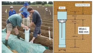
Figure 5. Installation of a fluxmeter into a field of potatoes (left), and the internal system of a fluxmeter showing the wick whose length L controls the suction at the soil interface, and the underlying reservoir to collect samples for analysis of leachate quality.
