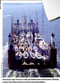
Dechou's Super Survivor 2-ship can ballast down and become a 'floating marina' into which yachts can sail to reserved positions
