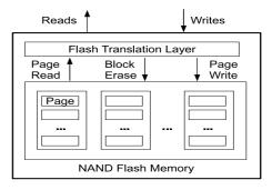
Figure 1: Internal architecture of a Solid State Drive (SSD)
