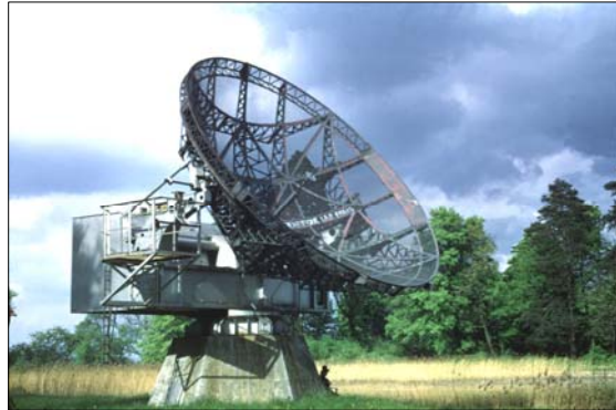
Figure 23: The 7.5m Würzburg antenna at Meudon Observatory (courtesy: Observatoire de Paris, Meudon).
