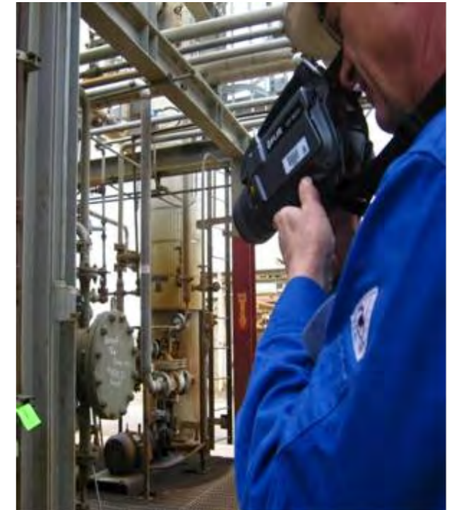
EPA inspector using an infrared camera to detect invisible organic chemical emissions.
