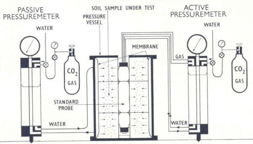
A pressure vessel, fitted with an internal expanding cylindrical membrane, is used with two pressuremeters for basic laboratory research on large samples, either of soil or other engineering materials such as asphalt, tarmac etc, and under rigorous temperature control if necessary.
