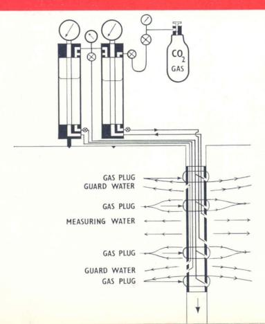
A double pressuremeter with a special probe squeezes water into a borehole at known pressures, and thereby measures the permeability of the ground at any desired depth, either above or below the water table. Guard cells neutralise end effects and air plugs at four places prevent leakage of water up or down the borehole.
