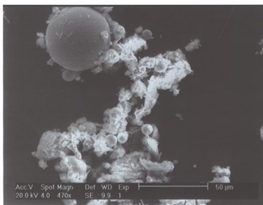
Figure 2. An SEM image from sample 2 shows a number of spherules along with other dust particles.
