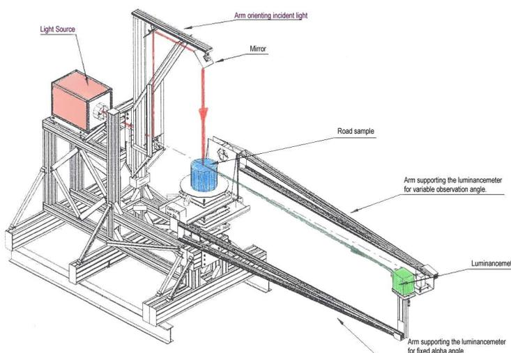
In this context, Schröder launched 3 years ago, in collaboration with the University of Liège, a research project called Memphis which aimed to improve the knowledge of road surfaces and overall to develop equipment capable of measuring the reflection characteristics of road surfaces on site.
