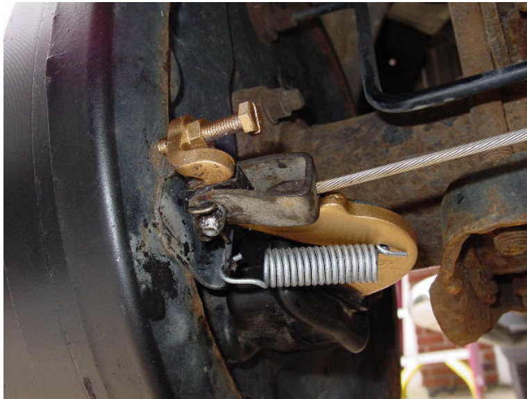
Fig. 18 Backside bellcrank installed
