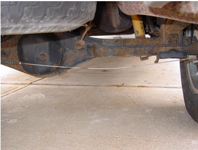
Fig. 1 Sagging park brake cable
