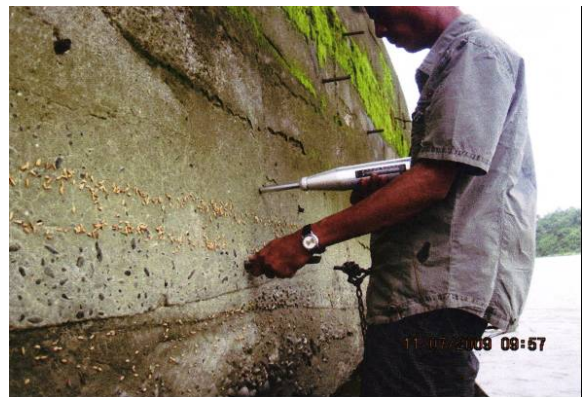
Photo-3.14 Survey using a Schmidt
