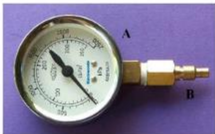
Fig Pressure gauge used to check if gas cylinder is full
