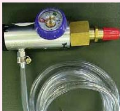
Fig 5.19: 6mm PVC tubing attached to MaxDog gas regulator
