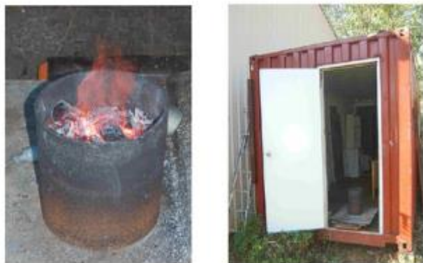
Fig 6.10. Charcoal burner brazier and test shipping container
