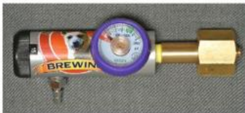
Fig: Max Dog Nitrogen flow regulator with pressure gauge to indicate if the cylinder is full and the click-flow setting (shown set to 15 litres/min)
