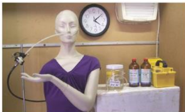
Fig 6.6. COGen 4 on fume cupboard test bench with acid bottles and CO monitor
