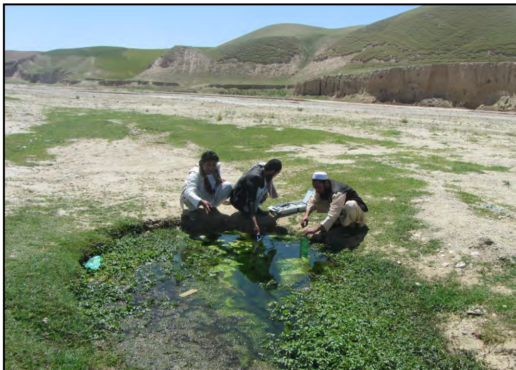
Figure 5.5. Kariz Qala spring emerging from the alluvial plain of the Maimana River in Pashtun Kot district around 10 km NW of Maimana city. Taken 5 th May 2013 by DACAAR. The discharge is around 2 L/s of water with an electrical conductivity of 1350 \mu\text{S}/\text{cm} .
