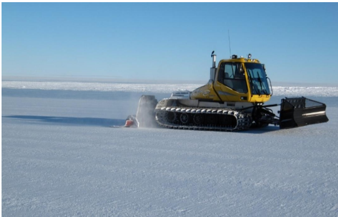
Image 2. A snow groomer tills the surface for greater friction and removes snow accumulation. Two of these machines will be based at the runway.
