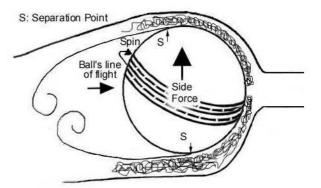
Figure 6. Schematic of flow over a cricket ball for reverse swing.
