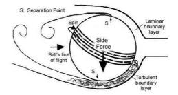
Figure 1. Schematic of flow over a cricket ball for conventional swing.
