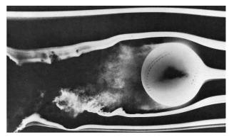
Figure 13. Smoke photograph of flow over a stationary (nonspinning) baseball. Flow is from right to left. Photograph by F.N.M. Brown, University of Notre Dame.
