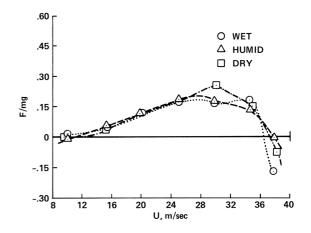
Figure 15. Effect of humidity on the measured side forces on a spinning cricket ball. Seam angle =  $20^{\circ}$ , spin rate = 5 revs/s.
