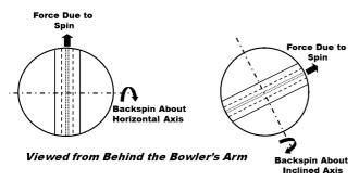
Figure 12. Schematic for spin-induced "Malinga" swing.
