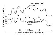
Figure 14. Surface contour plots of the primary seam on a cricket ball to investigate the effects of humidity.
