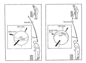
Figure 11. Spin bowlers using the Magnus effect to make the ball swing.
