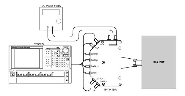
Setup 21. Test ID 8-6: TMDS - Intra-Pair Skew
