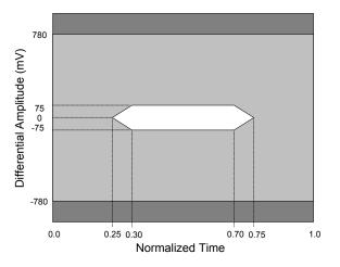
Figure 8-1 Absolute Eye Diagram Mask at TP2 for Sink Requirements
