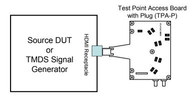
Figure 4-1 TPA-P, used for Source and Cable test calibration
