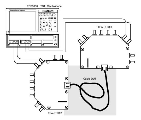
Setup 3. Test ID 5-5: Inter-Pair Skew
