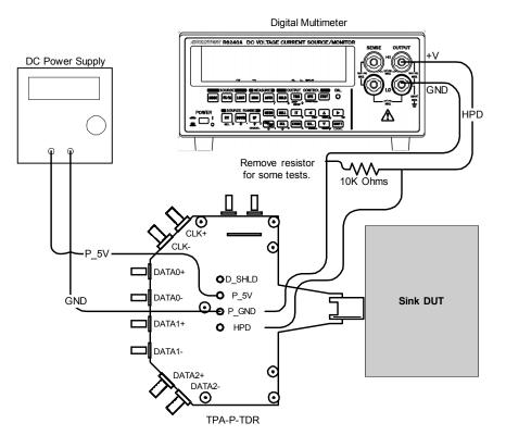
Setup 26. Test ID 8-11: HPD Output Resistance
