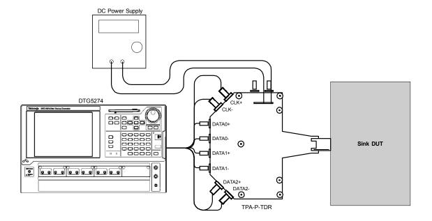
Setup 20. Test ID 8-5: TMDS – Minimum Differential Sensitivity
