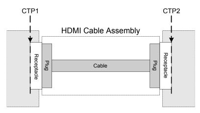
Figure 5-1 Cable Test Points
