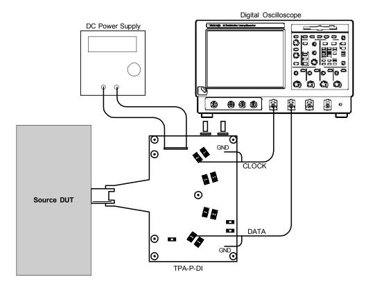
Setup 15. Test ID 7-10: TMDS – Data Eye Diagram
