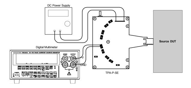
Setup 8. Test ID 7-3: TMDS – IOFF
