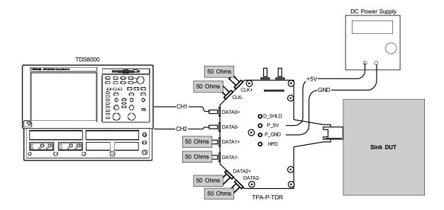
Setup 23. Test ID 8-8: TMDS – Differential Impedance
