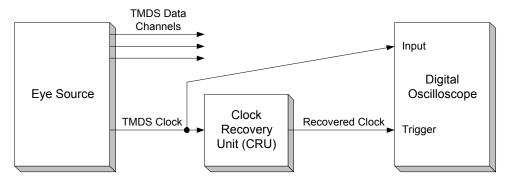
Figure 4-4 TMDS Clock Jitter Measurement: 1x clock output from CRU (pixel time)
