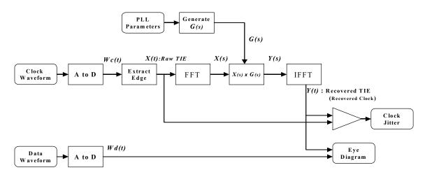
Fig.3 Proposed Clock Recovery Method
