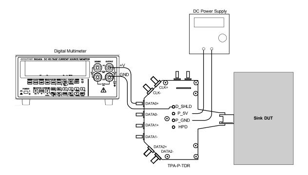
Setup 19. Test ID 8-4: TMDS - Termination Voltage
