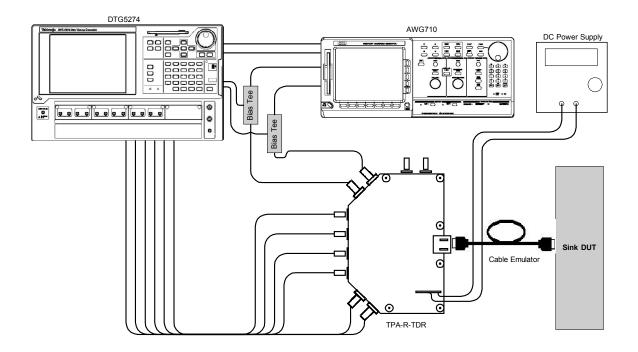
Setup 22. Test ID 8-7: TMDS – Jitter Tolerance
