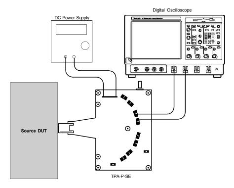
Setup 12. Test ID 7-7: TMDS – Intra-Pair Skew
