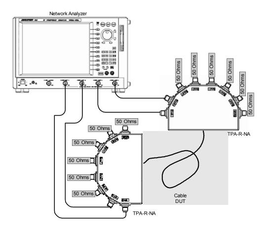
Setup 5. Test ID 5-7: Attenuation
