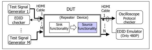
Figure 9-3 Testing of Source Functionality
