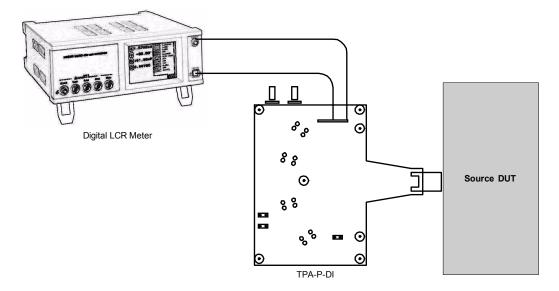
Setup 18. Test ID 7-13: DDC/CEC Capacitance
