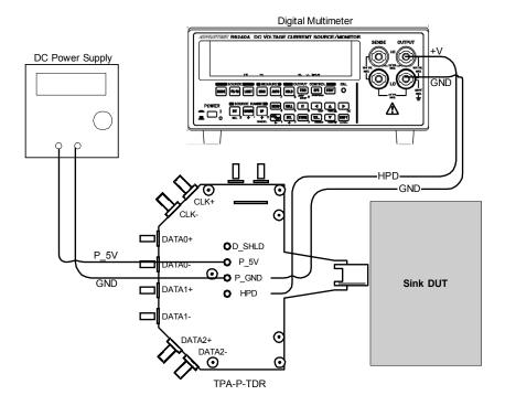
Setup 25. Test ID 8-10: HPD Output Voltage
