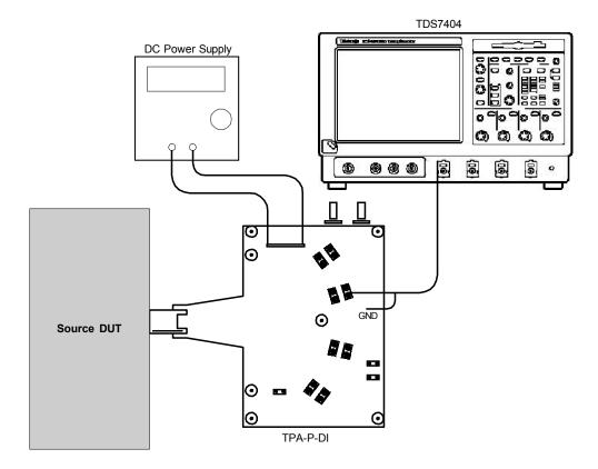
Setup 9. Test ID 7-4: TMDS – TRISE, TFALL
