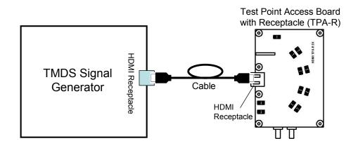
Figure 4-2 TPA-R, used for Sink and Sink test calibration
