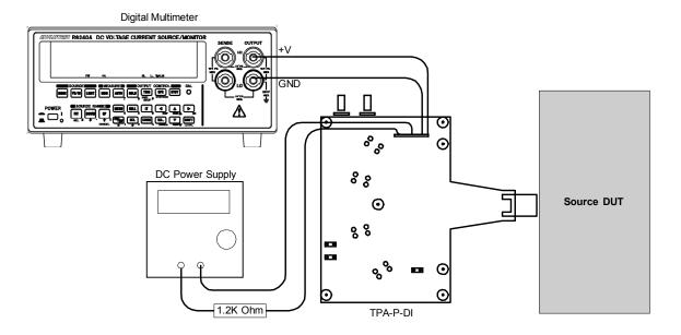
Setup 17. Test ID 7-12: Hot Plug Detect
