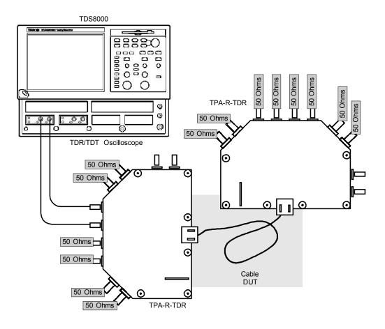
Setup 6. Test ID 5-8: Differential Impedance
