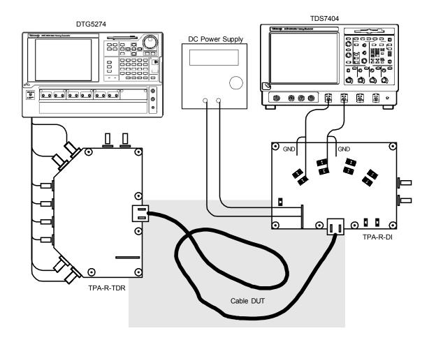
Setup 1. Test ID 5-3: TMDS Data Eye Diagram
