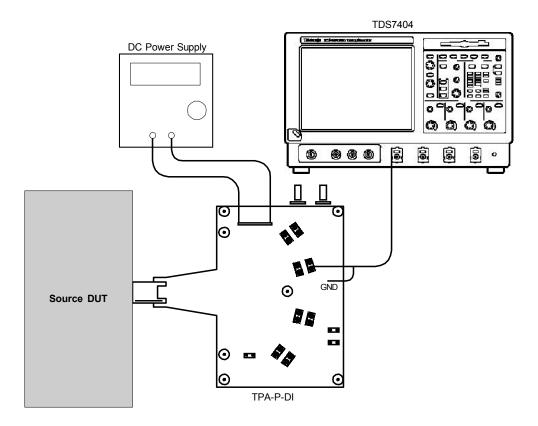
Setup 14. Test ID 7-9: TMDS – Clock Jitter
