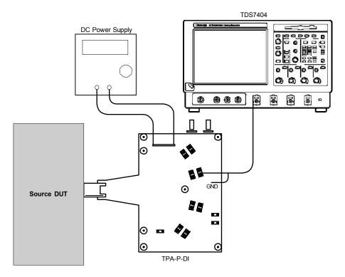
Setup 13. Test ID 7-8: TMDS – Clock Duty Cycle
