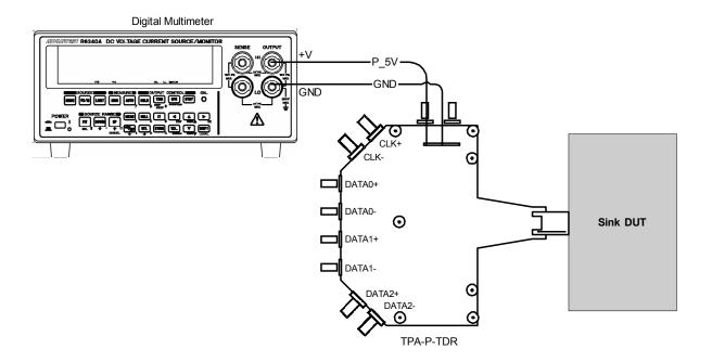
Setup 27. Test ID 8-12: +5V Power Max Current
