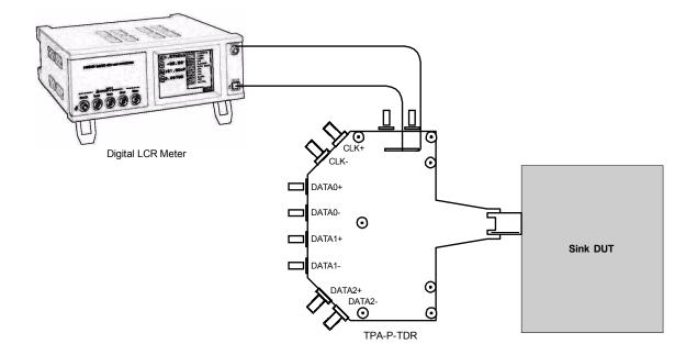
Setup 24. Test ID 8-9: DDC/CEC Line Capacitance
