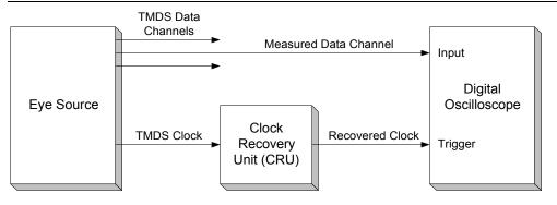
Figure 4-3 TMDS Eye Diagram Measurement: 10x clock output from CRU(bit time)
