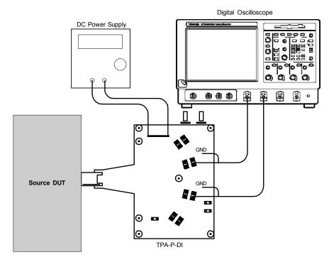
Setup 11. Test ID 7-6: TMDS – Inter-Pair Skew
