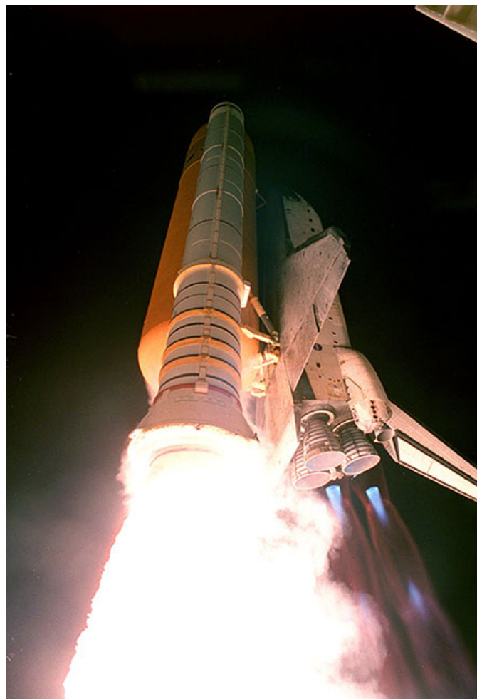
Fig. 2. Photograph of shuttle launch. Photograph shows blue color for \text{H}_2\text{-O}_2 fueled main shuttle engines (photo courtesy of NASA). (For interpretation of the references to color in this figure legend, the reader is referred to the web version of this article.)
