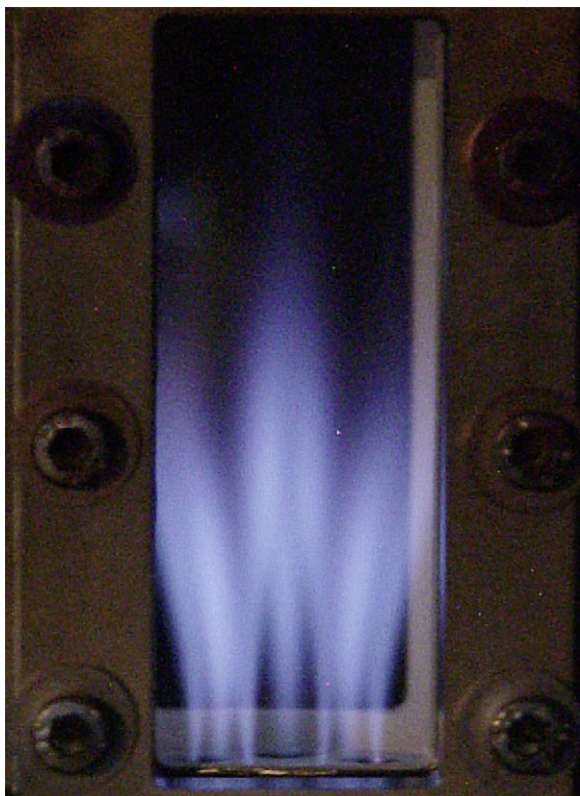
Fig. 1. Flame luminosity photograph in NASA Glenn hydrogen burner for inlet velocity of 90 m/s and \phi = 0.33 . Image taken at f/2.4 aperture with 0.6-s exposure time.
