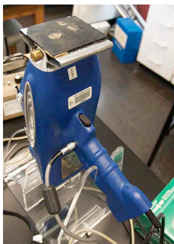
Figure 6: Each ambrotype was placed on the stage and analyzed with the portable XRF
