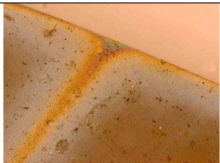
Figure 22: The white haze is due to the scattering of light by silver chloride crystals. The reddish orange tarnish is silver sulfide interference colors.
