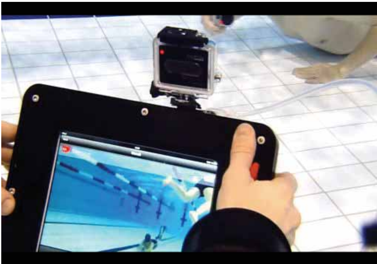
Figure 2. Pool testing GoPro Hero3™ video camera with a wireless connection to Apple iPad™.
