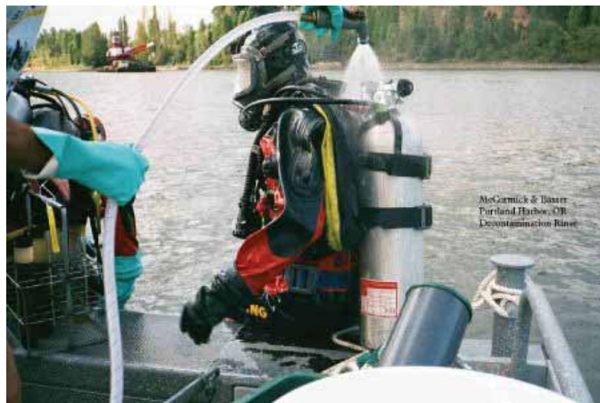
Figure 10. ERT diver undergoing potable water decontamination at the McCormick and Baxter portion of the Portland Harbor Superfund Site. The Region 10 and ERT divers were collecting contaminated bottom sediment cores for lab analysis. Photo by B. Duncan.
