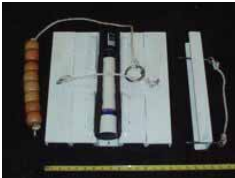
Figure 2. Pressure sensor assembly.
