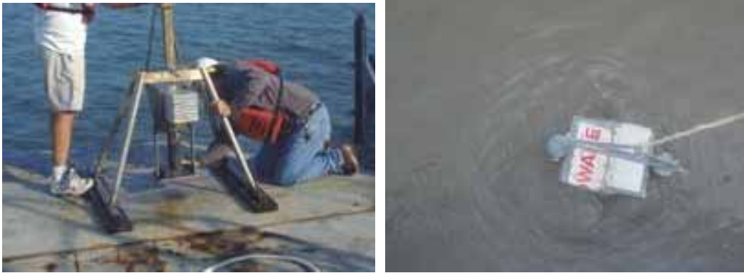
Fig. 6. (a) above, shallow sediment corer, (b) right, a sediment grab deployed at Jekyll Creek, AIWW.
