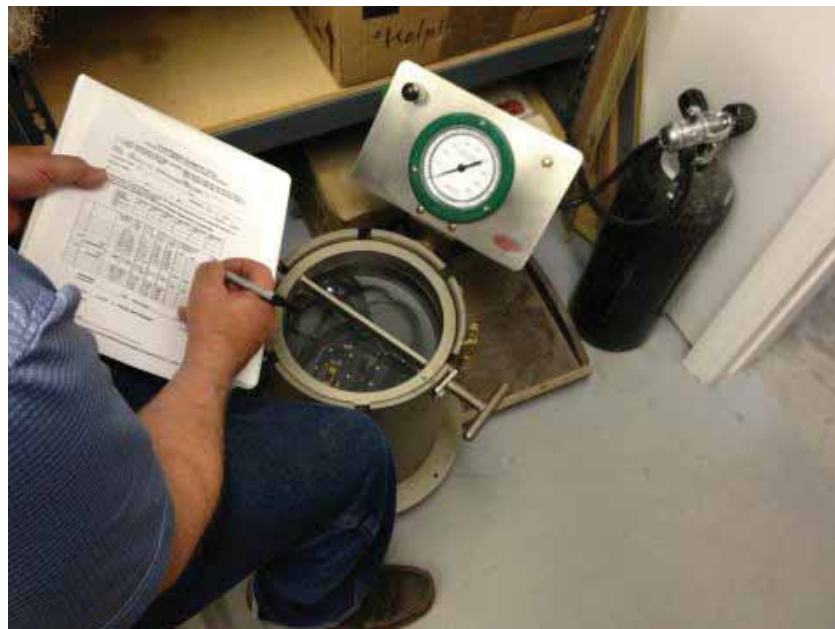
Figure 2. CCR head in pressure pot for test run on sensor and computer performance
