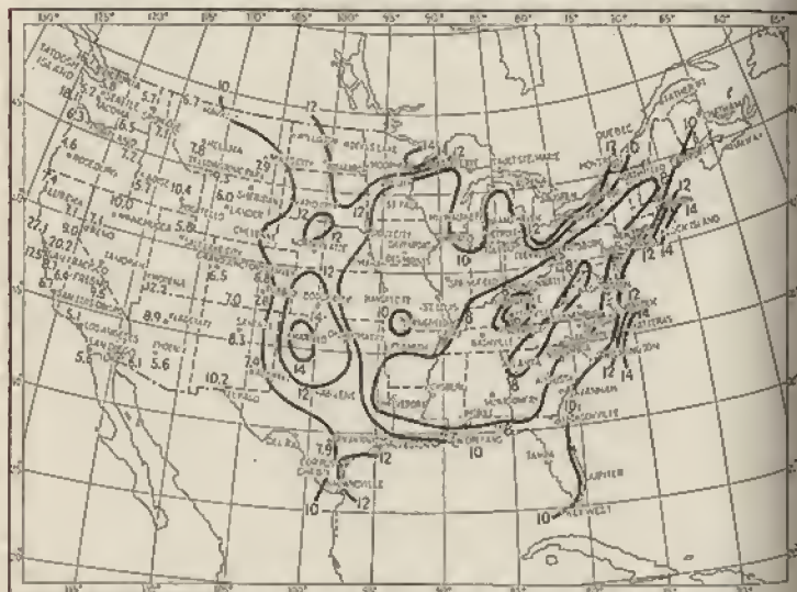
FIG. 11.—Average hourly velocity of the wind for an elevation of 100 ft. (Courtesy of Weather Bureau, U. S. Department of Agriculture.)
