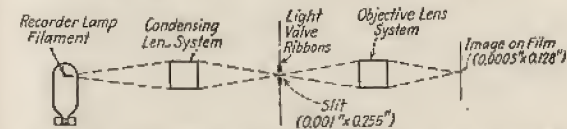
FIG. 38.—Optical system used in light-valve recording.
