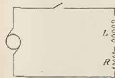
FIG. 3.—Series circuit containing resistance and inductance.
