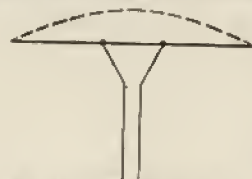
FIG. 35.—Method of connecting line to radiator.
