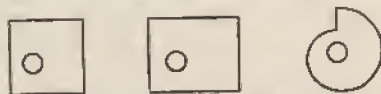
FIG. 27.—Irregular baffle shapes used outdoors to broaden frequency band of destructive interference between speaker front and back waves at listener's position.
