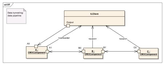
Figure 3-4. Example of Data Tunneling Among OpenMAX Components
