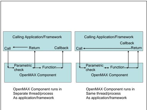
Figure 2-5. Out-of-Context versus In-Context Operation
