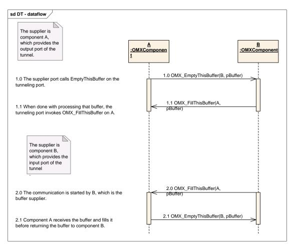
Figure 3-10. Data Flow Between Tunneled Components
