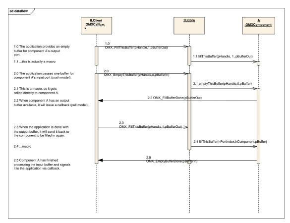
Figure 3-9. Data Flow Between Non-tunneled Components
