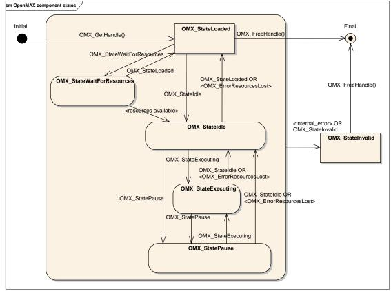
Figure 3-2. OpenMAX Component State Transitions
