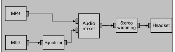
Figure 4-1. Audio Payback Processing Chain
