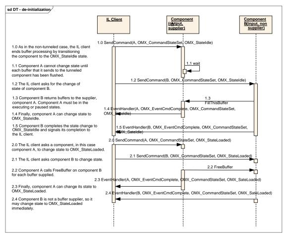
Figure 3-13. De-initialization of Tunneled Components
