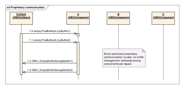
Figure 3-11. Data Flow with Proprietary Communication Between Components
