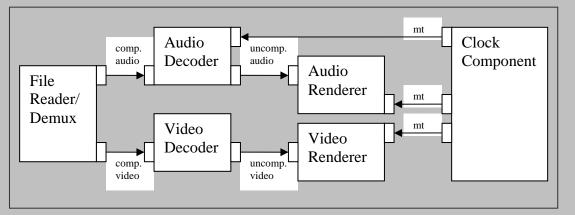
Figure 6-4. Example Use Case of Audio-Video File Playback
