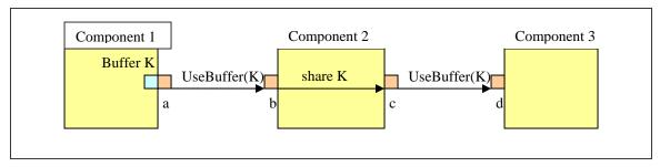
Figure 2-6. Example of Buffer Allocation and Sharing Relationships
