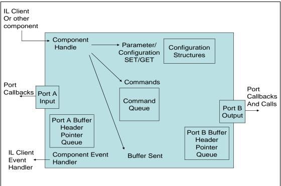
Figure 2-4. OpenMAX IL API Component Architecture
