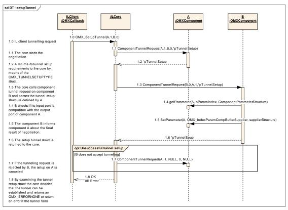
Figure 3-5. Tunnel Setup
