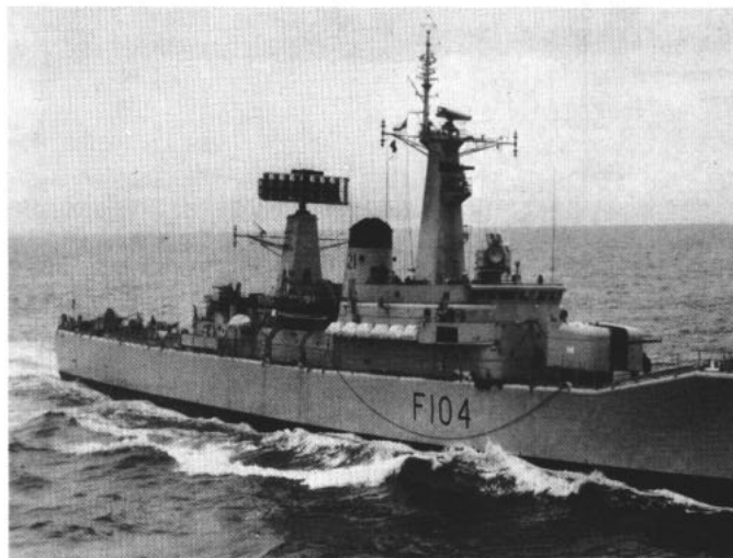
United Kingdom General purpose frigate HMS Dido (F104), commissioned in 1963, is equally able to engage surface ships, aircraft and shore batteries as well as ASW assignments. She is armed with triple-barreled ASW mortar, a twin 4.5 inch mortar and two 40-mm AA guns aft. A Wasp copter with torpedoes extends her ASW punch.
