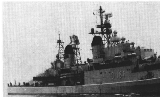
Federal German Navy Federal German Navy destroyer Hamburg (DD 181) was commissioned in 1964 and recommissioned after refitting in 1969. Hamburg is 440 feet long and is armed with four 100-mm turrets, four 40-mm antiaircraft guns, torpedo tubes and medium range antisubmarine rocket launchers.
