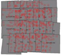
Figure 6a: Graphic overview of the block layout with GCPs, check points and automatically collected tie points
