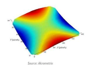
The encapsulation layer has a thermal expansion coefficient (CTE) higher than those of other constituents is formed on both lateral sides and upper sides of the dies, thus the die package warps, thereby deteriorating the reliability of the die package.
