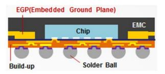
The **EGP**, typically fabricated from copper, is used to control warpage of the panel assembly, but also the die shift and can also be used to provide a single routing option for ground in a finished semiconductor package.
