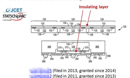
An insulating layer disposed over the die (and encapsulant) and into a channel formed in the die and/or encapsulant.
